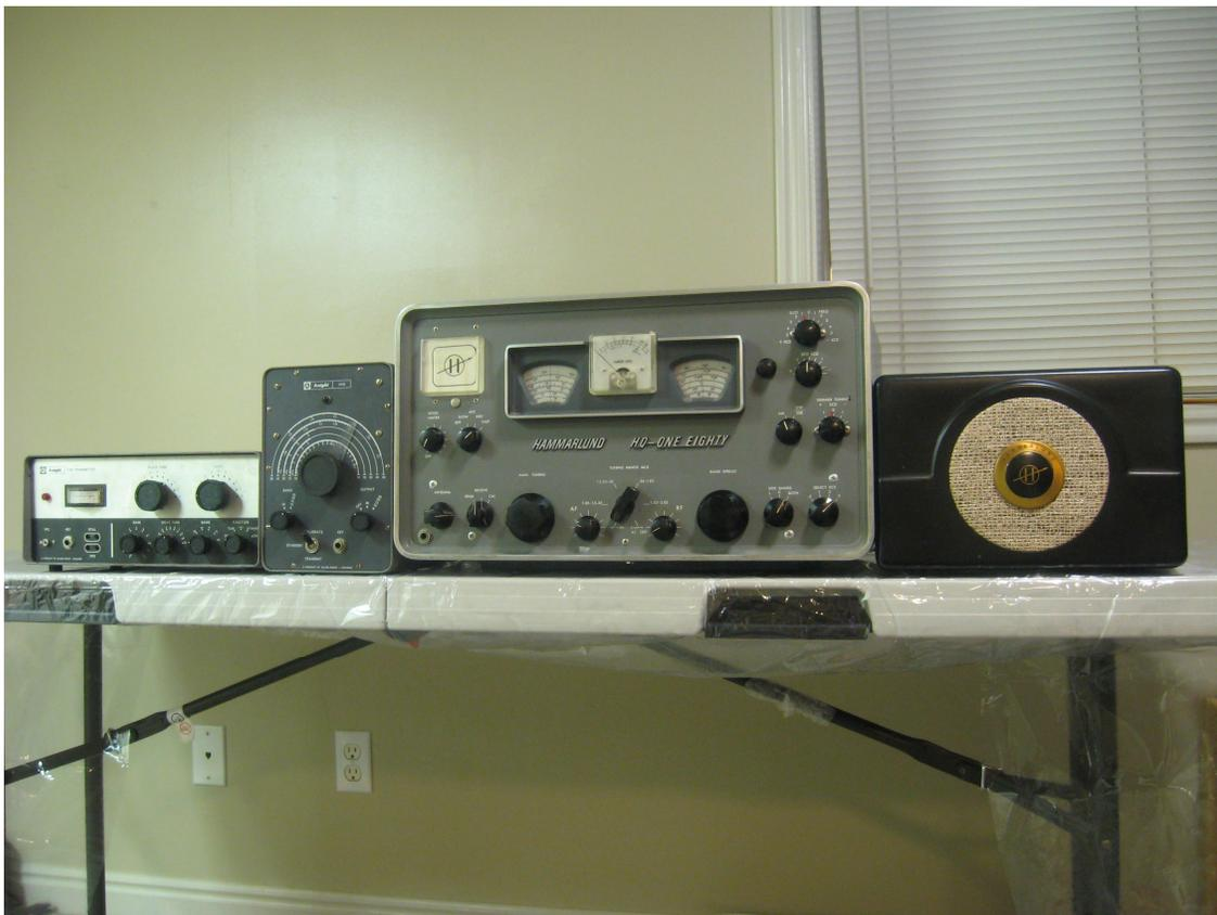
The picture, provided by Jason, above shows the beginning of a nice classic station in his ham shack. The AM-CW transmitter on the left is a Knight T-60. The variable frequency oscillator (VFO) is a V44. As an aside, the transmitter and VFO have a Knight logo on them, but in the manuals they are Knight Kits.
