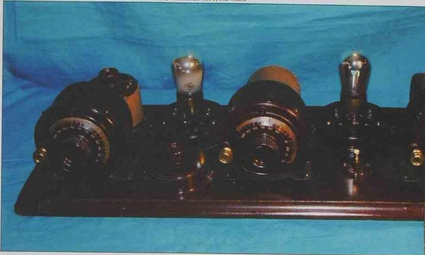
▲ During the early 1900s, "breadboard" radios similar to this were often made at home by radio enthusiasts. Pictured here is a commercial breadboard radio manufactured by Atwater Kent in 1924.
