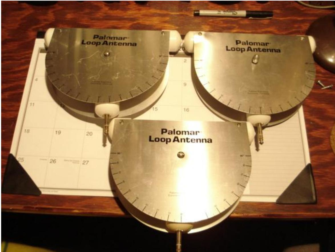
The loop amplifier is powered by a nine-volt battery. A red Light Emitting Diode shows that the power is on. I have to keep a fresh battery on hand in case I forget to turn it off. I use my Kenwood PS-2000 receiver to directly tune those frequencies. They go down to an indicated 30 KHz on the dial, but it is advertised to start at 50 KHz. I can copy WWVB National Bureau of Standards at 60 KHz. The radio covers continuously through the Broadcast Band and higher.
