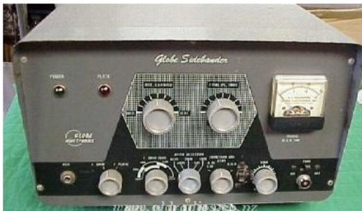
DSB 100 Double-sideband transmitter. It put out 50 watts on CW, 40 on AM and 100 on DSB no carrier.
