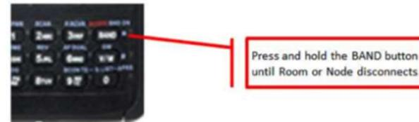
Figure 90 FT1D and FT1XD Disconnect method
