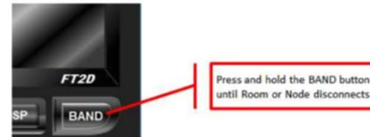
Figure 91 FT2D Disconnect methods
