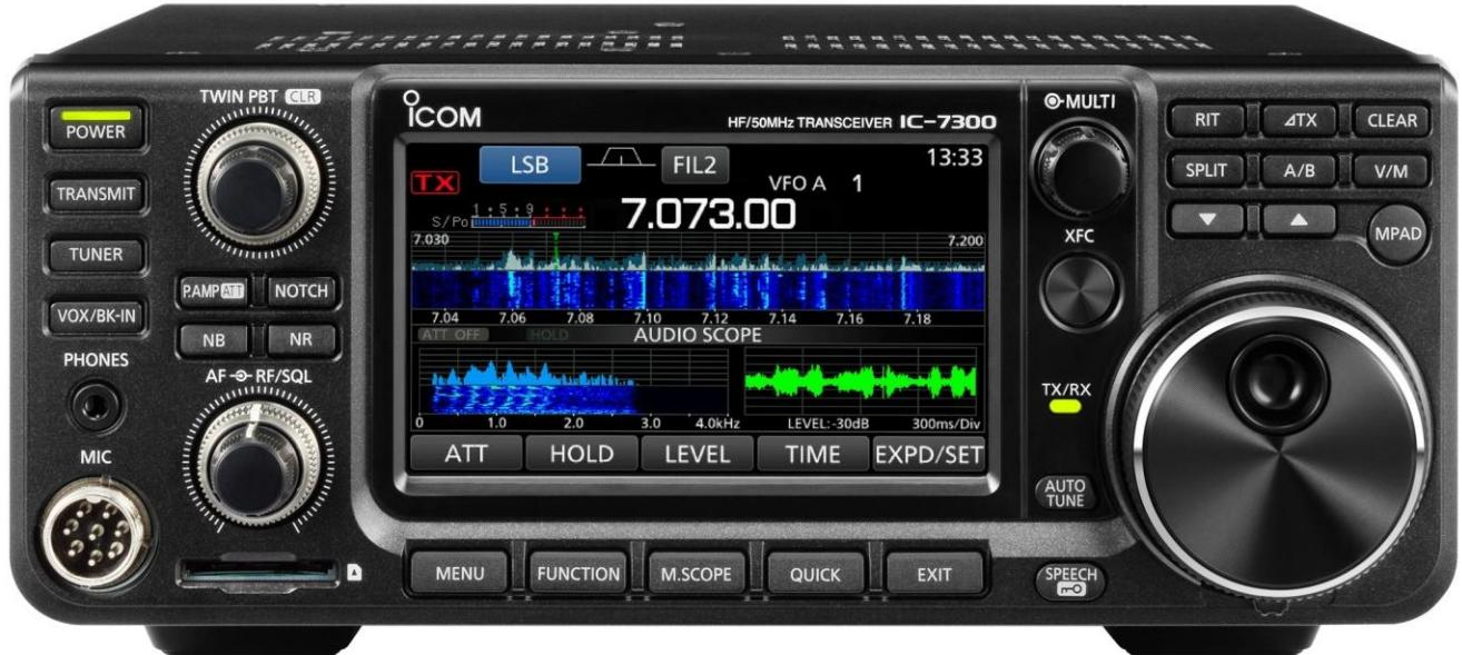
The ICOM IC-7300 is an HF + 6 meter, multi-mode, self-contained Software Defined Radio (SDR) transceiver with knobs, buttons and a touch screen. It also has a real-time spectrum display with pan adapter and water fall displays.
