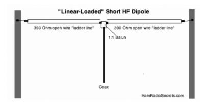
This page describes a way to build a linearly-loaded dipole antenna with a feedpoint impedance of approximately 35  $\Omega$ . This allows you to feed it with coax instead of the ladder line that I use. The author uses 390  $\Omega$  ladder line for the elements. He says it's commonly available, but I don't think I've ever seen 390  $\Omega$  ladder line. You could probably use 450  $\Omega$  ladder line by adjusting the element lengths a little.
