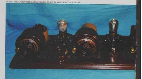
▲ During the early 1900s, "breadboard" radios similar to this were often made at home by radio enthusiasts. Pictured here is a commercial breadboard radio manufactured by Atwater Kent in 1924.
