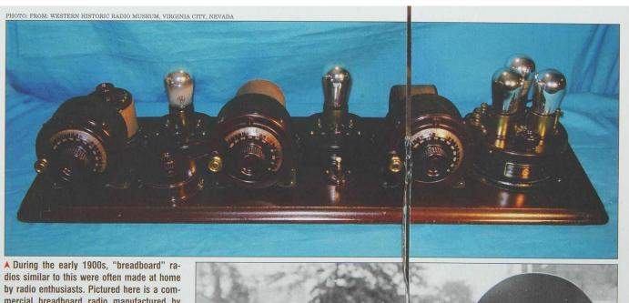
mercial breadboard radio manufactured by Atwater Kent in 1924.
