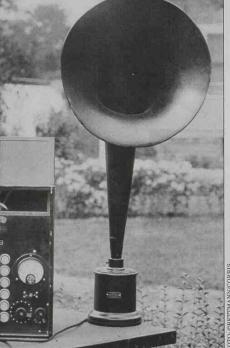
▲ This rather elaborate radio using a horn speaker is probably homemade and dates from around 1922.
