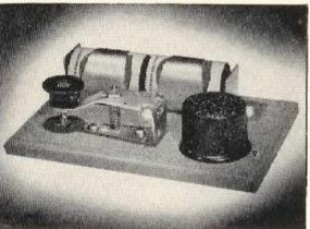
Make a modern version by using a "piezo buzzer" and a nine volt battery. The key is made from a door "strap" hinge. The parts list is as follows:
