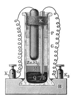
The **Clark cell**, invented by English engineer <u>Josiah Latimer Clark</u> in 1873, is a <u>wet-chemical cell</u> (colloquially: *battery*) that produces a highly stable <u>voltage</u>. In 1893, the output of the Clark cell at 15 C was defined by the International Electrical Congress as 1.434 volts, and this definition became law in the United States in 1894. This definition was later supplanted by one based on the Weston cell. [1]
