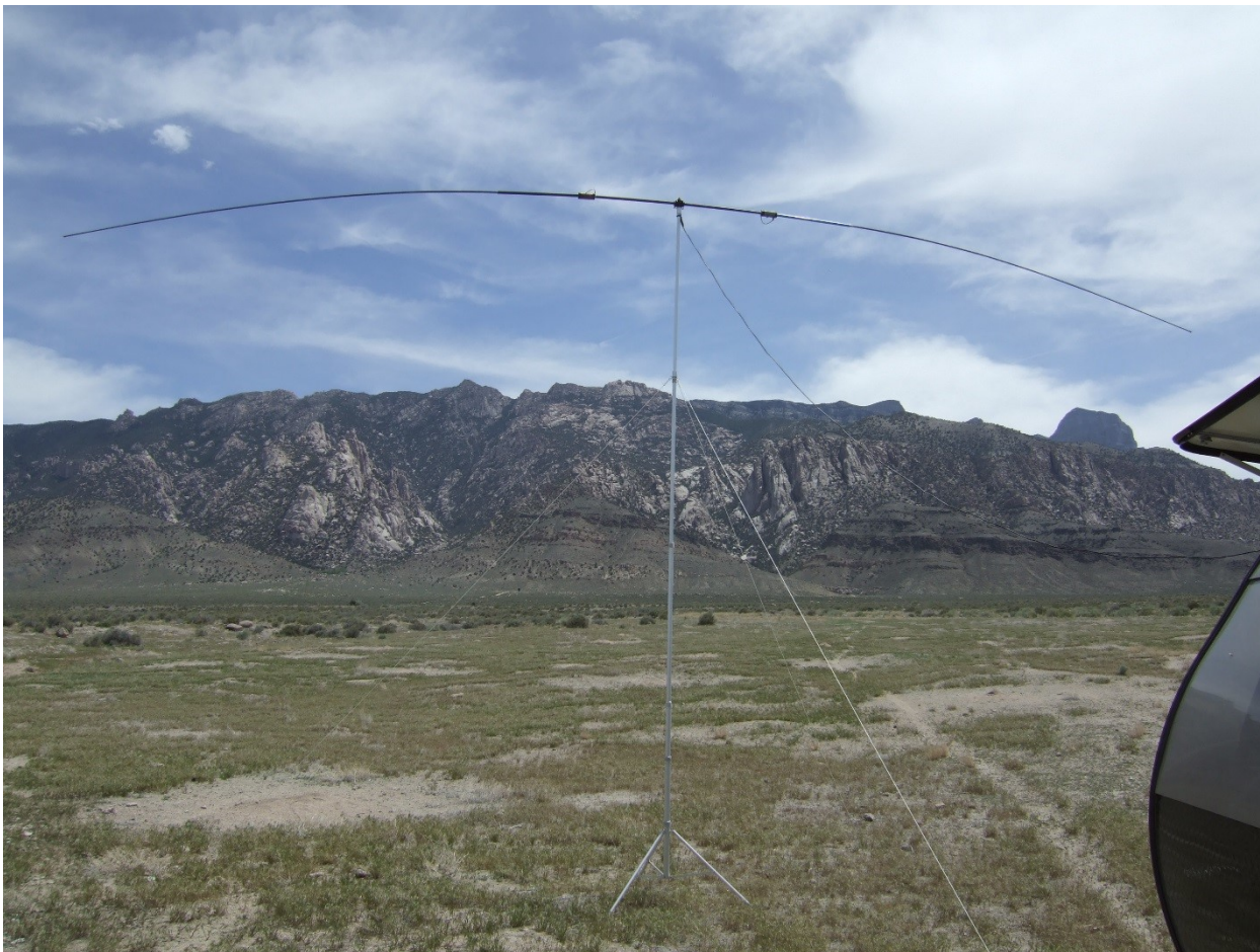
Figure 3 Buddi Pole in a dipole configuration with taps on the coils for quick 20 and 40 meter band changes.
