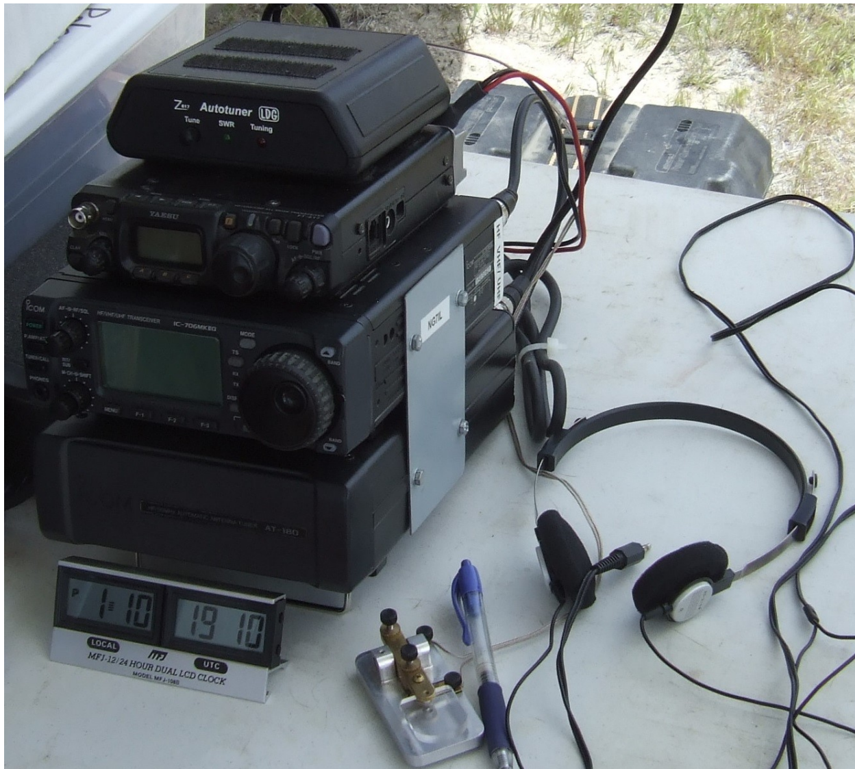
Figure 1 Icom 706MKII with auto tuner, FT817 and tuner for QRP, and a portable lightweight straight key.
