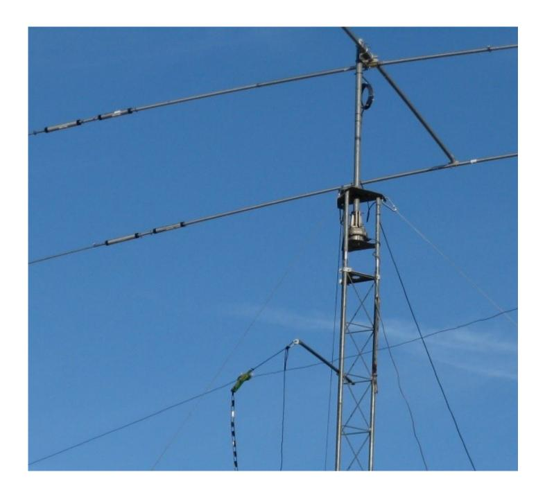
This antenna was tied to a balanced tuner and was capable of operating on all the HF bands. It really worked well on 40 meters as it had gain which improved our ability to hear and be heard.
